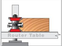
6) Using multiple passes, the stile cuts can now be made.
