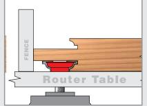
**4)** With the assistance of the fence, make several passes to create the extended tenon.
