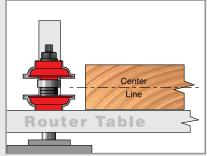
**1)** Install the rail bit and vertically center the bit with the stock.
