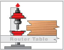
**3**) While leaving the rail bit in place, remove the top section of the router bit.
