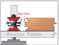
**5)** Install the stile cutter bit and align the top of the groove cutter to the top of the tongue of rail cut.
