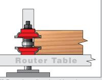
2) Rout the rail ends with stub tenons.
